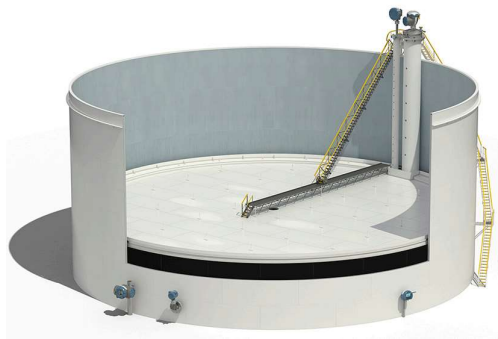
Floating roof tank
