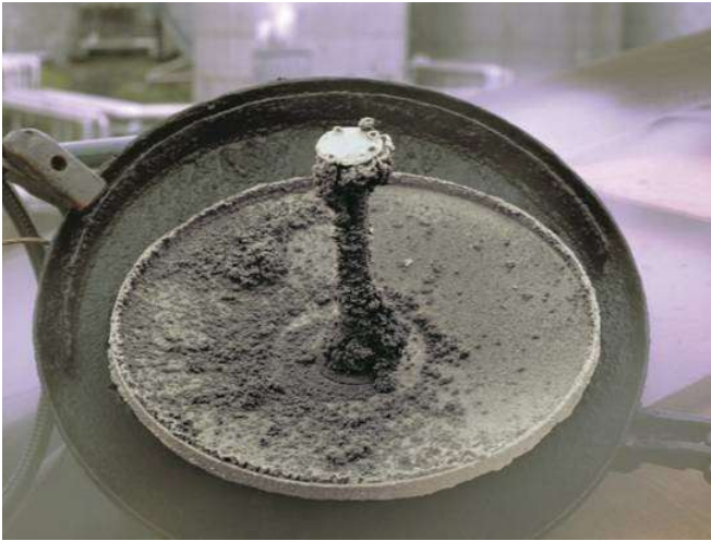
The antenna is in operation after having been exposed to blown bitumen at 220 °C (430 °F) for several months.
