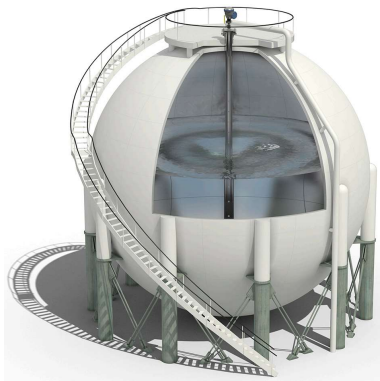
Pressurized LPG tank
